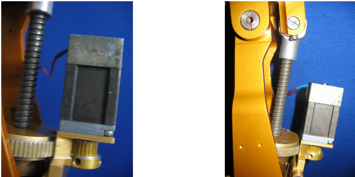
Picture 6. Motor drive with ball-screw mechanism
