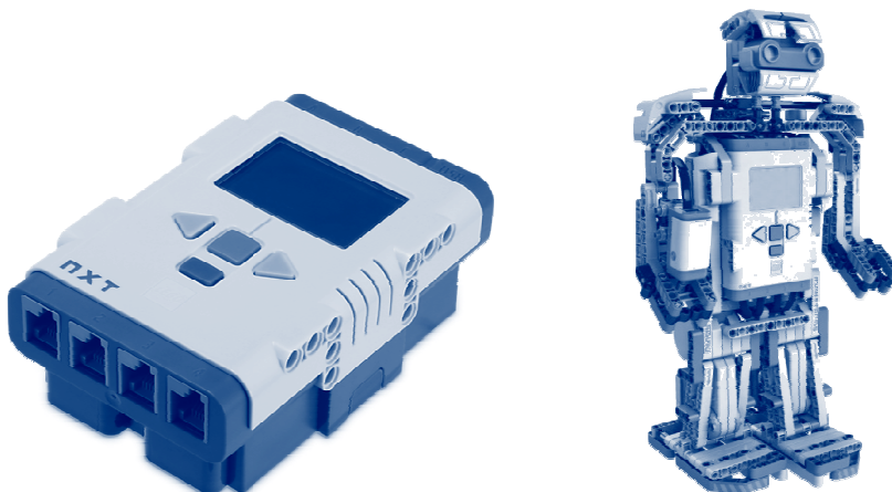
Figure 3.3. The NXT Intelligent Brick (left) and the most common humanoid robot configuration-Alpha Rex (right)
