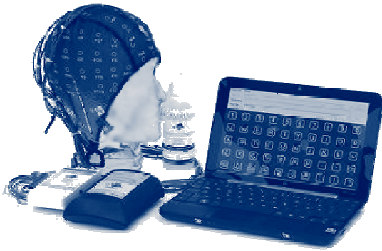
Figure 2.2. Noninvasive BCI, equipment for P300 speller
