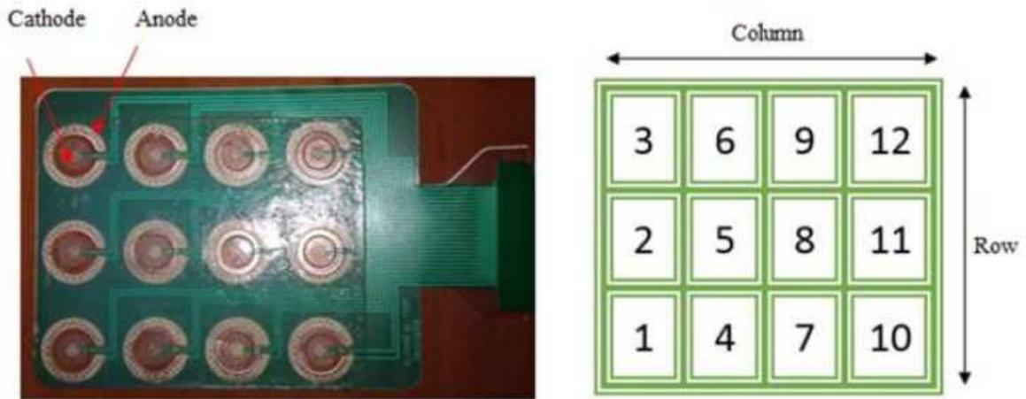
**Figure 8.** The matrix with 12 concentric electrodes (left) and the sketch of the annotation of the fields on the matrix (right).
