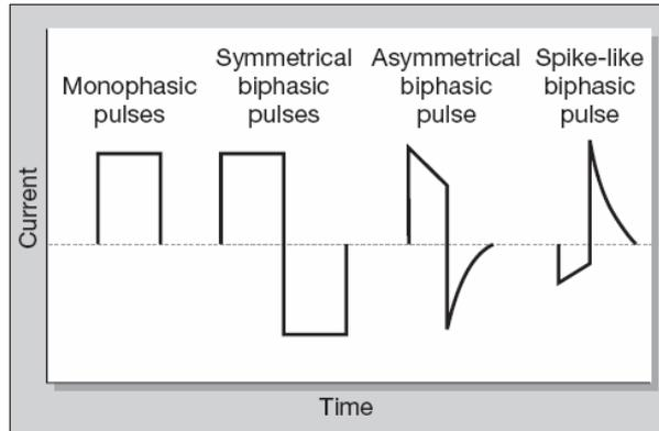
***Figure 7. Typical signal shapes for TENS [1]***
