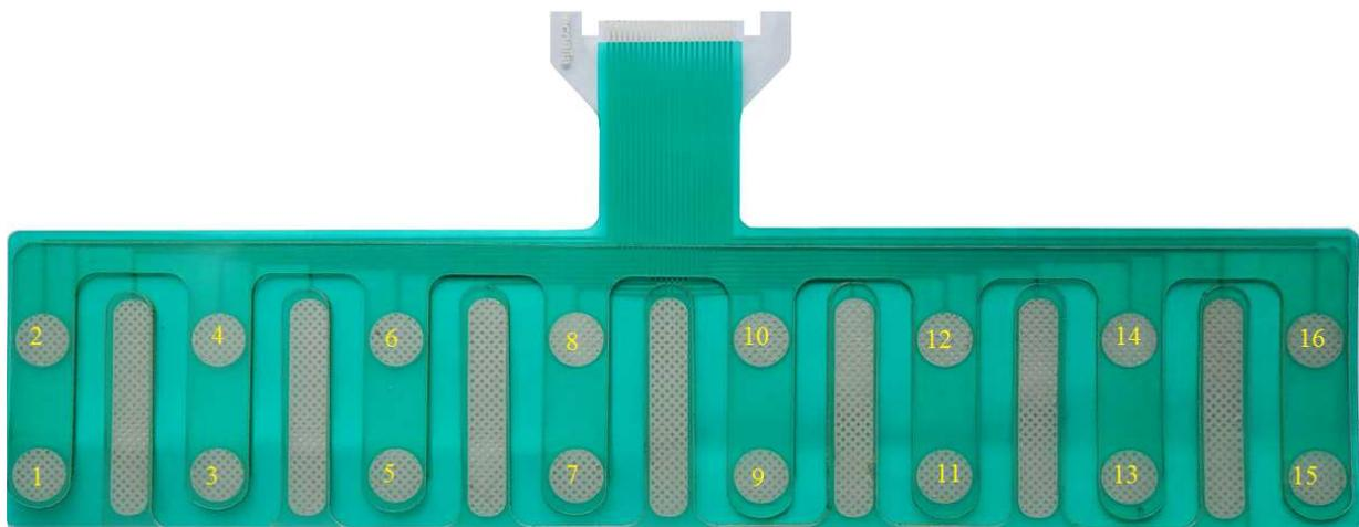
*Figure 13 The new configuration of the multipad electrode for afferent stimulation.*
