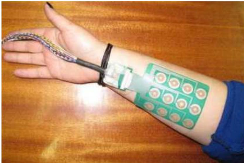
***Figure 10. The matrix with 12 electrodes positioned on the forearm for measurements.***
