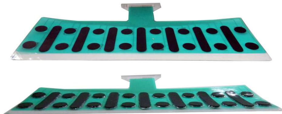
***Figure 14. Multipad electrodes used, coated with a thin (up) and thick (down) layer of conductive rubber.***
